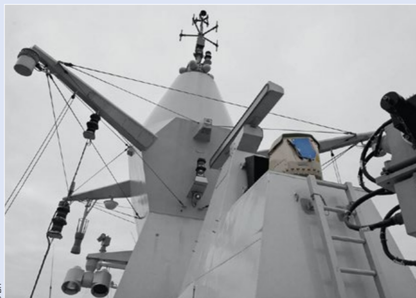
Système de veille infrarouge VAMPIR NG. VAMPIR NG InfraRed Search and Track (IRST).
